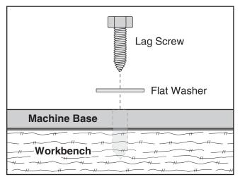
Figure 10. Example of a direct mount setup.
